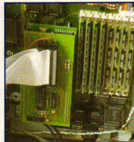
Sitting comfortably in this well-endowed machine, the NOVA extends the Falcon's graphic capabilities considerably.
