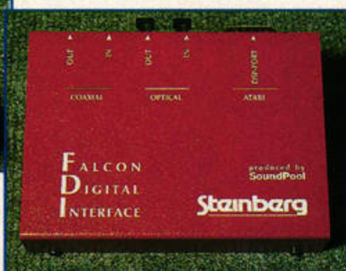
The Falcon Digital Interface is a fibre optic and coaxial digital link with your DAT machine or other digital gear. It enables you to back up your hard drive to DAT and access your DAT machine's AD converter.
