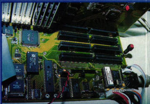
The Eagle bus in action, with the bottom three slots free and the RAM card on top.
