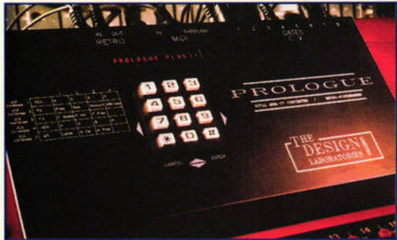
The Prologue-2 takes MIDI input and converts it to the old CV and GATE system, bringing a new lease of life to your analogue synthesisers.
